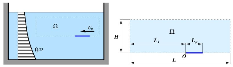
The dimensions are set to L = 1.5 m, H = 0.5 m,  $L_i = 1.0 m$ ,  $L_p = 0.025 m$ . The grid has  $258 \times 117$  points with the minimum cell size in the near-wall region  $\Delta z = 0.5 mm$
