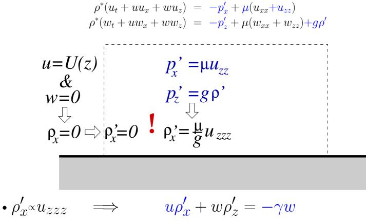
• inlet velocity profile generates vertical velocity perturbation
