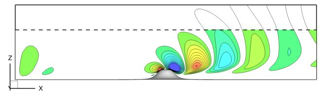
**Vertical velocity contours in the plane of symmetry** – *truncated domain* –  $\frac{\partial p}{\partial n} = 0$ .
