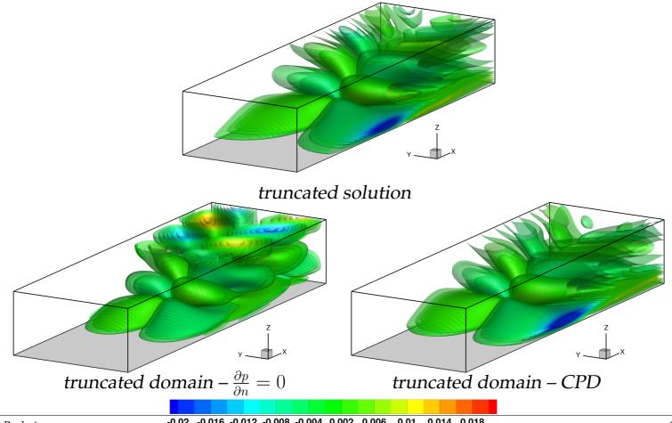
**Isosurfaces of the vertical velocity component** w - nondimensionalized  $\tilde{w} = w/U_*$ .
