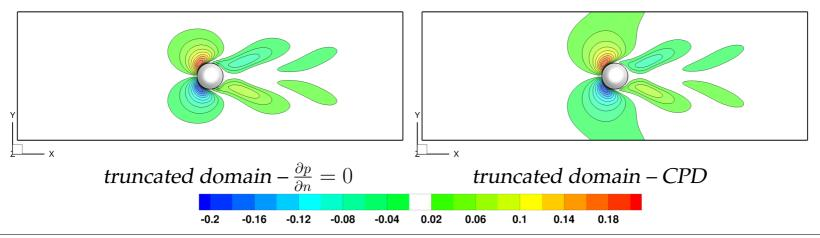
**Isosurfaces of the transversal velocity component** v - nondimensionalized  $\tilde{v} = v/U_*$ .
