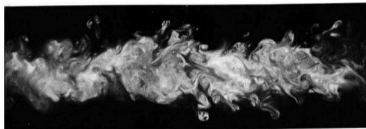
174. Turbulent wake of a cylinder. A sheet of laser light slices through the wake of a circular cylinder at a Reynolds number of 1770. Oil fog shows the instantaneous flow pattern, covering 40 diameters centered 50 diameters downstream. Photograph by R. E. Fuku
